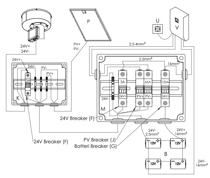
The solar panels (P) and AC connection (U) must be installed by a certified electrician. However, the preparation work may be done by a layman as long as local code requirements are followed. Please read the solar station's user manual for additional information on how to install and configure the station.
