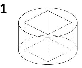
Make a hole for the concrete at your chosen location. The hole for a PV-6 should be at least 80x80 cm, 1 m deep (~600 liter). Refer to the manual for more information.
