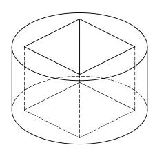
Make a hole for the concrete at your chosen location. The hole for a PV-6 should be at least 80x80 cm, 1 m deep (~600 liter).
