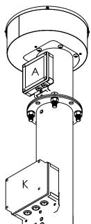
If the string inverter and 24VDC transformer is placed away from the solar installation the junction box (K) can be wired as shown above.
