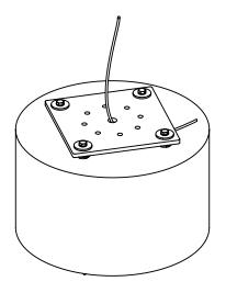
Pull a strong wire through the center hole of the base plate and out through the hole beneath the junction box on the foundation column.
