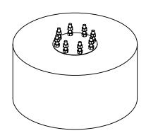
Fill the holes 2/3 full with chemical anchor adhesive (400-500 ml). Push the rod unit into the holes and give the adhesive time to cure before continuing the assembly.
