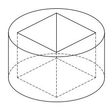
Make a hole for the concrete at your chosen location. The hole for a PV-6 should be at least 80x80 cm, 1 m deep (~600 liter).
