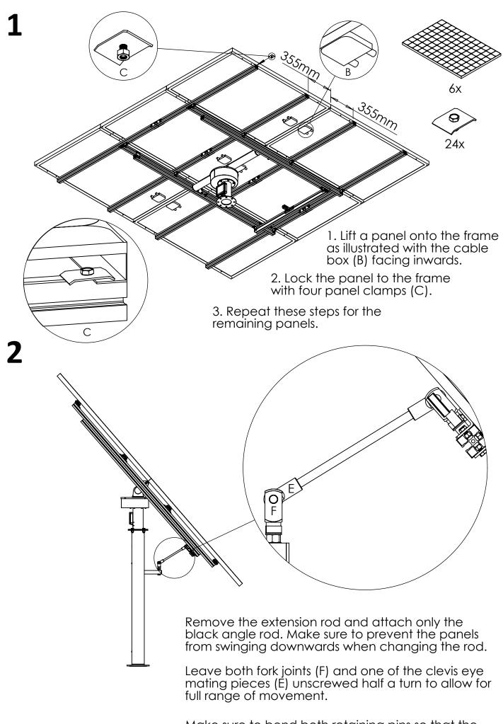
Make sure to bend both retaining pins so that the fork joint bolts are held in place.
