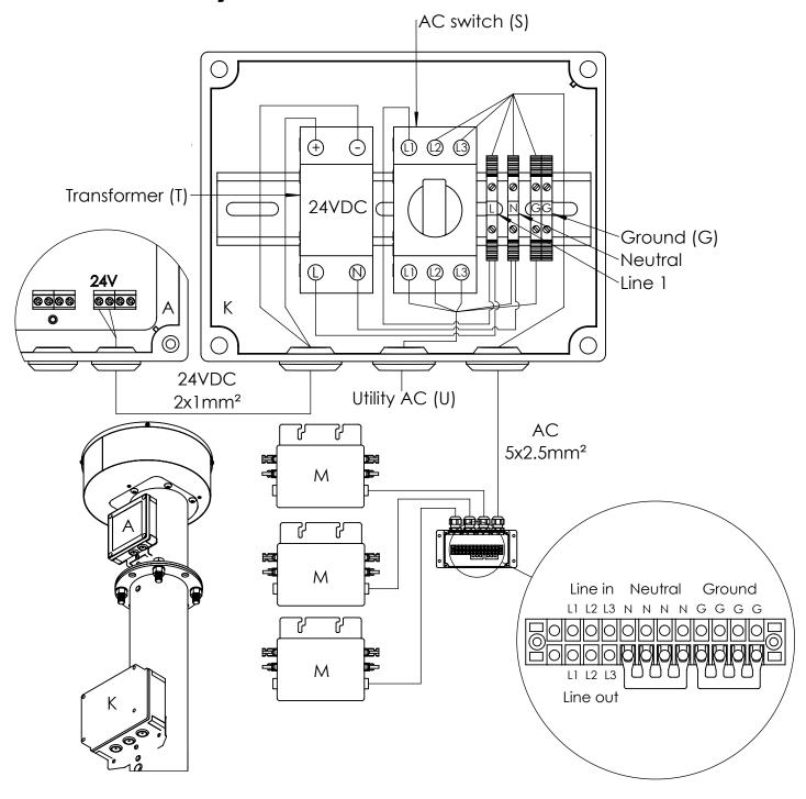
The PV solar panels, microinverter (M) and utility AC (U) must be connected by a certified electrician. However, preparation work may be done by a layman as long as local code requirements are followed.
