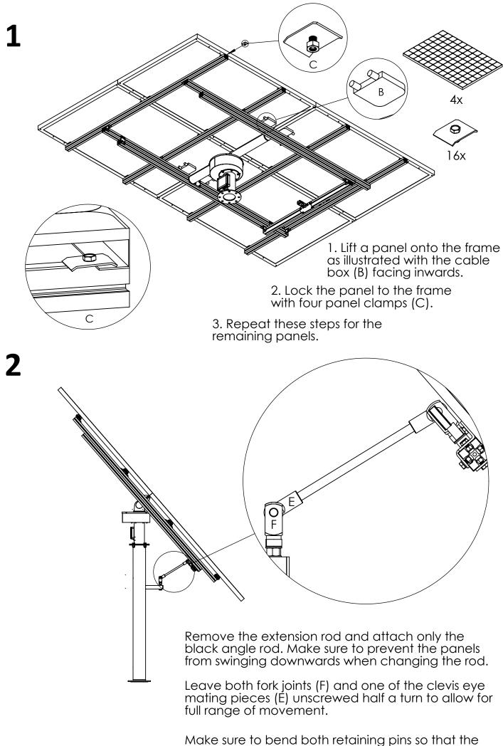
Make sure to bend both retaining pins so that the fork joint bolts are held in place.
