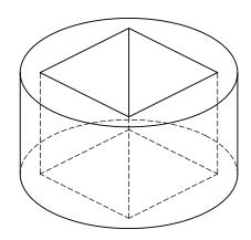
Make a hole for the concrete at your chosen location. The hole for a PV-4 should be at least 70x70 cm, 80 cm deep (~400 liter).
