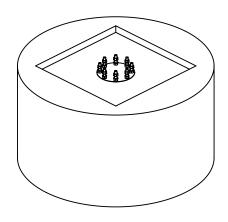
Push the rod unit into center of the concrete and let the flange rest on top of the concrete. Use a spirit level to align the flange horizontally.
