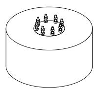
Fill the holes 2/3 full with chemical anchor adhesive (400-500 ml). Push the rod unit into the holes and give the adhesive time to cure before continuing the assembly.
