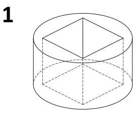
Make a hole for the concrete at your chosen location. The hole for a PV-4 should be at least 70x70 cm, 80 cm deep (~400 liter).
