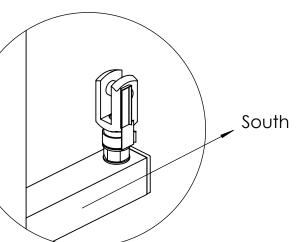
1. Mount the column including the bottom flange on the rod unit as illustrated.
