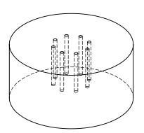
Drill eight holes vertically into the bedrock using the rod unit as a template. Make the holes 20 mm wide and 250 mm deep. Use compressed air to remove any debris and water from the holes to ensure a clean bonding surface.
