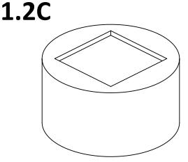
Fill the hole with concrete up to ground level.
