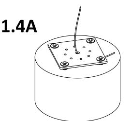
Pull a strong wire or the cable through the center hole of the base plate and out through the hole beneath the junction box on the foundation column.
