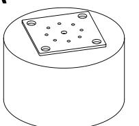
Place the base plate on level ground and use it as a template to mark the positions for the ground anchors.
