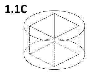
Make a hole for the concrete at your chosen location. The hole for a PV-3 should be at least 65x65 cm, 70 cm deep (~300 liter).
