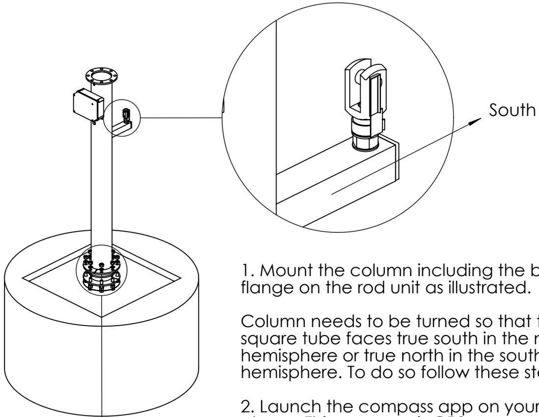
1. Mount the column including the bottom flange on the rod unit as illustrated.
