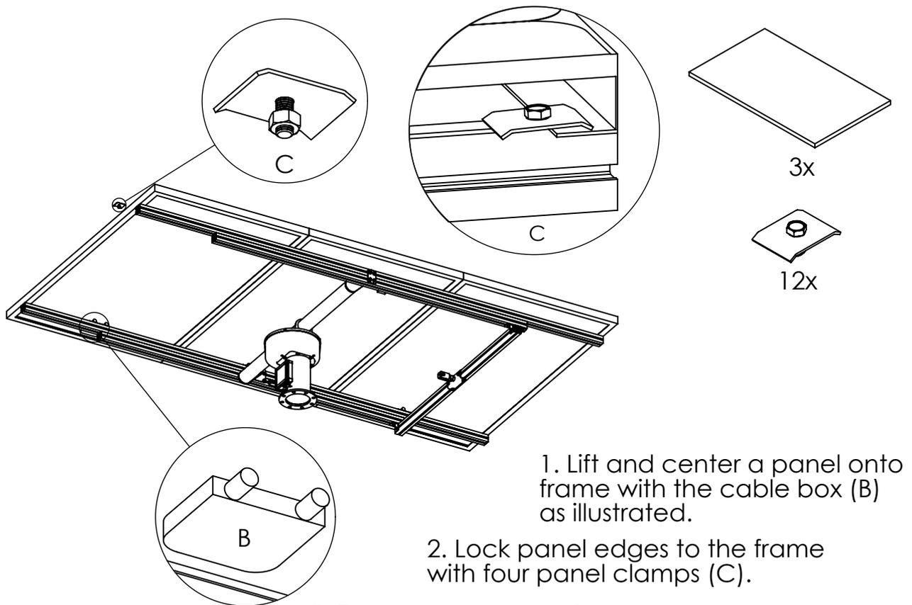
1. Lift and center a panel onto frame with the cable box (B) as illustrated.
