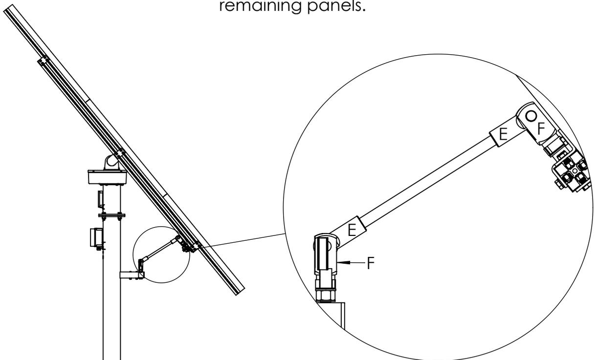
Remove the extension rod and attach only the black angle rod. Make sure to prevent the panels from swinging downwards when changing the rod.
