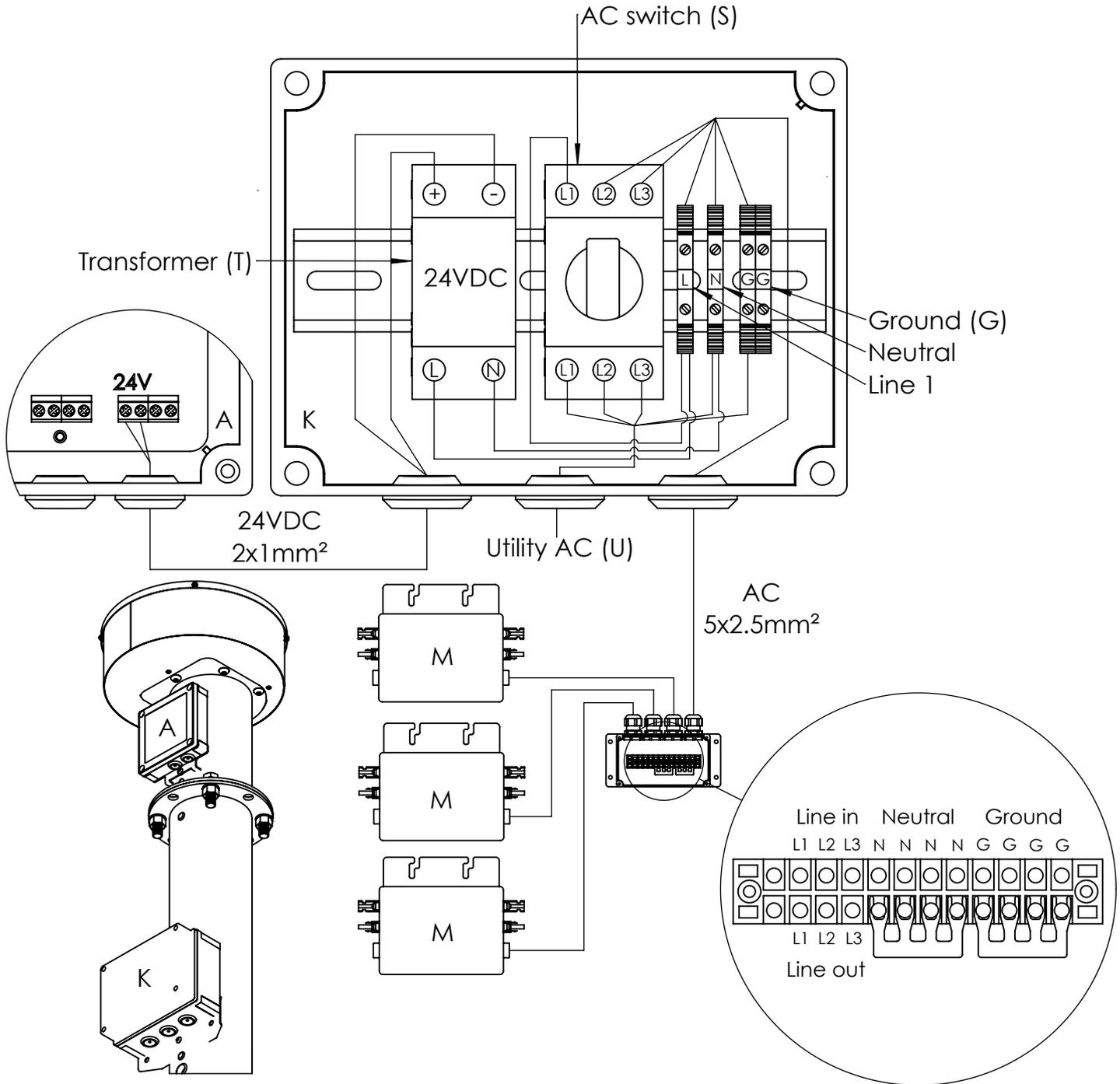
The PV solar panels, microinverter (M) and utility AC (U) must be connected by a certified electrician. However, preparation work may be done by a layman as long as local code requirements are followed.
