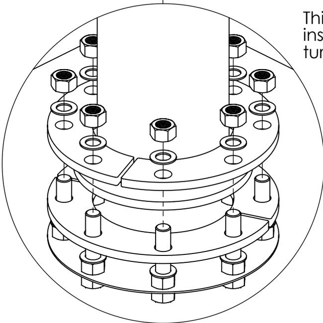
5. Adjust bottom nuts to horizontally align the column's upper flange using a spirit level.
