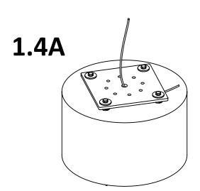
Pull a strong wire or the cable through the center hole of the base plate and out through the hole beneath the junction box on the foundation column.
