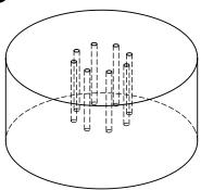
Drill eight holes vertically into the bedrock using the rod unit as a template. Make the holes 20 mm wide and 250 mm deep. Use compressed air to remove any debris and water from the holes to ensure a clean bonding surface.
