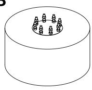
Fill the holes 2/3 full with chemical anchor adhesive (400-500 ml). Push the rod unit into the holes and give the adhesive time to cure before continuing the assembly.
