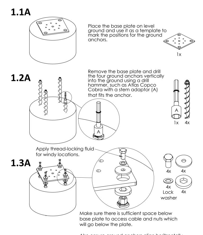
Also ensure ground anchors align horitzontally using a spirit level. Then attach base plate using the fastening elements.
