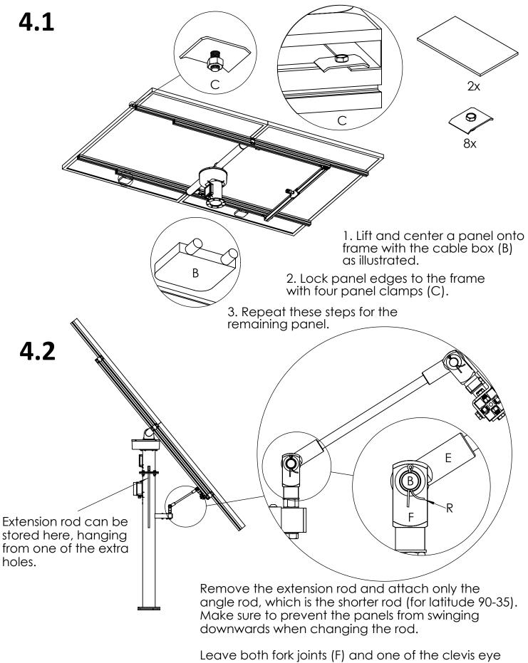
mating pieces (E) unscrewed half a turn to allow for full range of movement.
