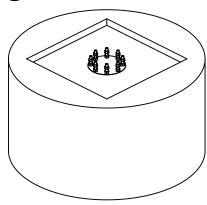
Push the rod unit into center of the concrete and let the flange rest on top of the concrete. Use a spirit level to align the flange horizontally.
