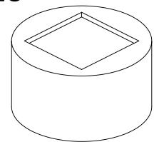
Fill the hole with concrete up to ground level.
